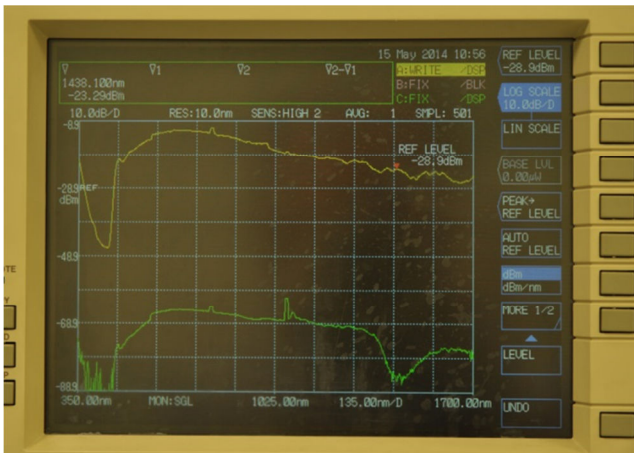
Fig. 3 – Graph of measurement taken in the sprague dawley rat sciatic nerve shown by Spectrum Analyzer display.
