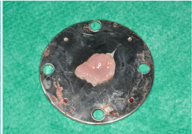
Fig. 2 – Sprague dawley rat muscle vision (sample 2) positioned on the plate. The part thickness of 0.3 mm is positioned on the central hole.
